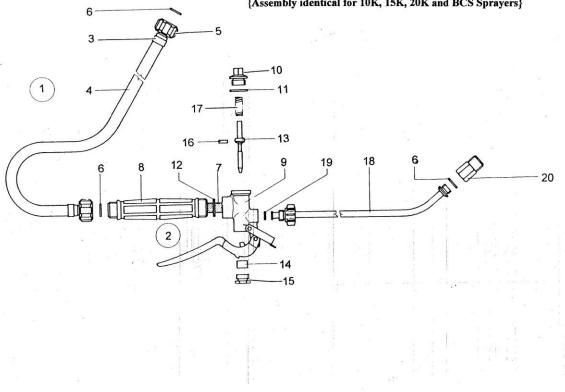
Hose, Valve, and Wand Assembly Parts
